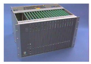
outputs. Each video matrix switching control unit has RS-422 data communication port. Provides camera title, 24 hour time/date, monitor number and titling displays can be selected by 8 step of grey scale.
